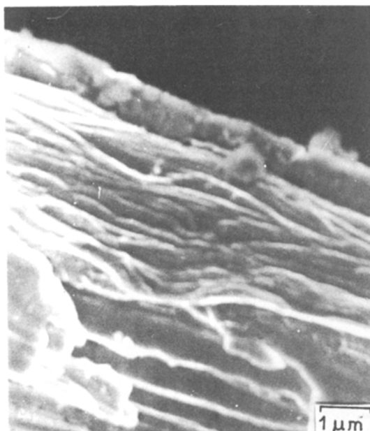
Figure 14 Fracture surface obtained by repeated bending of a Zr-33 at% Ni ribbon. Long ridges running across the width of the specimen can be seen.
